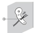
**6** Reconnect the detached speaker cords, matching  $\oplus / \odot$  to the appropriate speaker terminals (1), and then push the lever down completely (2).
